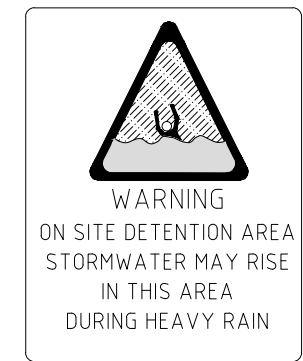
OSD WARNING SIGN NTS
